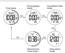
If the watch is not under time mode, the display will return to time mode when button S3 is pressed after press either button S1 or S2
